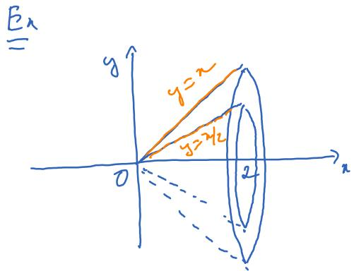
Each cross section is an annulus. At position  $x$ , the inner radius is  $\frac{x}{2}$  and the outer radius is  $x$ .
