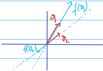
Every vector on the line parallel to  $v_1$  (which we denote by  $\mathbb{R}v_1$ ) is scaled by factor 2. Every vector on the line parallel to  $v_2$  (which we denote by  $\mathbb{R}v_2$ ) is scaled by factor -1.
