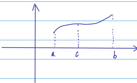
$$\int_a^c f(x) dx + \int_c^b f(x) dx = \int_a^b f(x) dx$$
