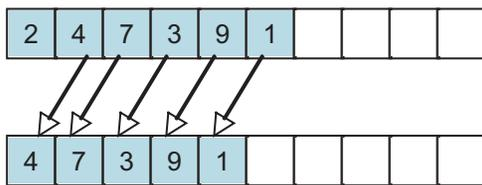
Removing a value requires elements to slide left. Sliding left means every element must be moved, and hence is an  $O(n)$  operation.
