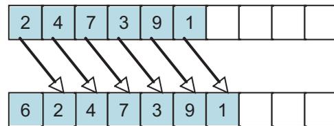
This does not mean that a *Dynamic Array-like* data structure cannot be used to implement a queue. The key insight is that we can allow the starting location of the block of elements to “float”, rather than being fixed at location zero. An internal integer data field records the current starting location.
