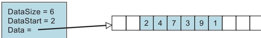
Notice that the “logical” index no longer corresponds to the physical index. The value with logical index zero is found in this diagram at array location 2. The value with logical index 1 is found at location 3, and so on.
