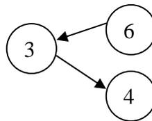
The solution is to first perform a rotation on the child, and then rotate the parent. This is termed a *double rotation*.
