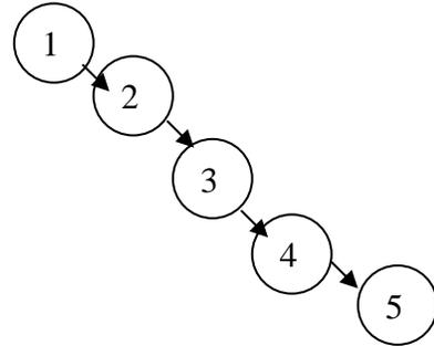
To preserve fast performance we need to ensure that the tree remains well balanced. One way to do this is to notice that the search tree property has some flexibility. Three nodes that are unbalanced can be restored by a *rotation*, making the right child into the new root, with the previous root as the new left child. Any existing left child of the old right child becomes the new right child of the new left child. The resulting tree is still a binary search tree, and has better balance.
