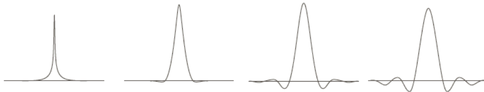
FIGURE 4.46 (a)–(d) Spatial representation of BLPFs of order 1, 2, 5, and 20, and corresponding intensity profiles through the center of the filters (the size in all cases is 1000 \times 1000 and the cutoff frequency is 5). Observe how ringing increases as a function of filter order.
