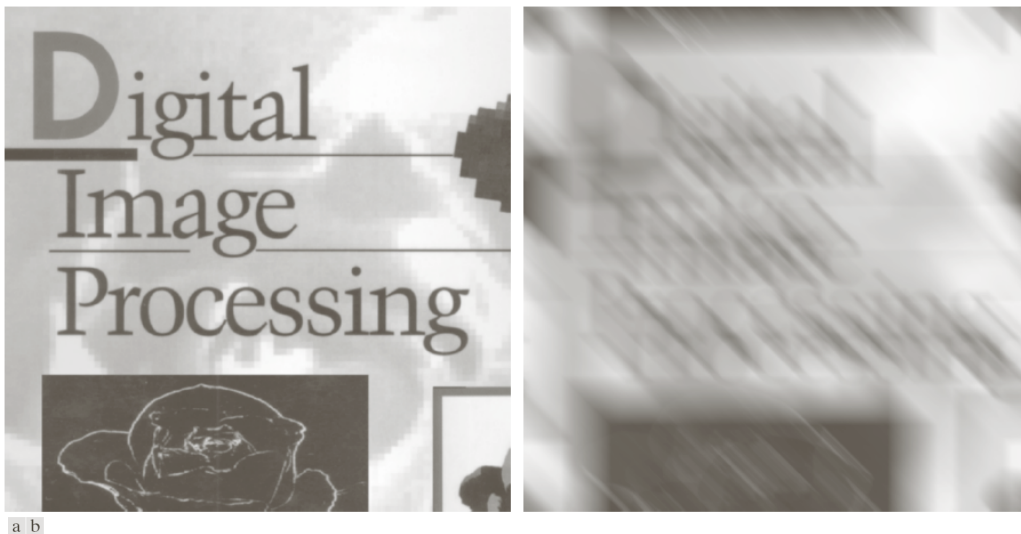
a b FIGURE 5.26 (a) Original image. (b) Result of blurring using the function in Eq. (5.6-11) with a = b = 0.1 and T = 1 .
