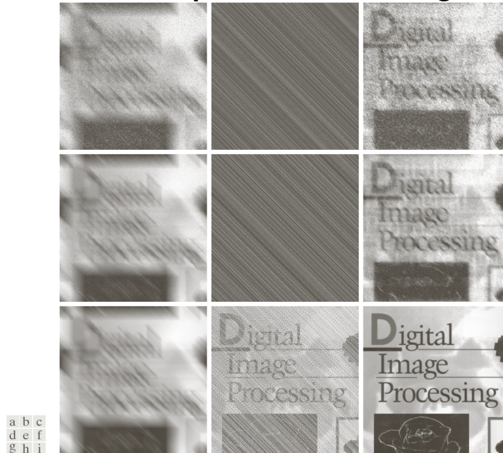
FIGURE 5.29 (a) 8-bit image corrupted by motion blur and additive noise. (b) Result of inverse filtering. (c) Result of Wiener filtering. (d)–(f) Same sequence, but with noise variance one order of magnitude less. (g)–(i) Same sequence, but noise variance reduced by five orders of magnitude from (a). Note in (h) how the deblurred image is quite visible through a “curtain” of noise.
