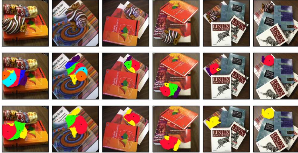
Fig. 5. DTSTBN-based image segmentation: invariance across translation, rotation and scaling. (top row) 256 \times 256 images; (middle row) pixel clusters with the same parent at level 3; (bottom row) pixel clusters with the same parent at level 4; points mark the position of parent nodes.
