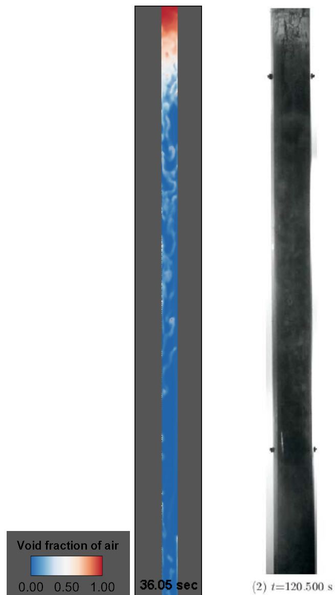
Figure 4.7: Simulation B3, L_v=6m and V_{air}=1.703 m^3 , flow snapshots in the vertical pipe at t = 36.05 s (numerical simulation) and t = 120.500 s (physical experiment of Leon (2018) under the same system conditions).
