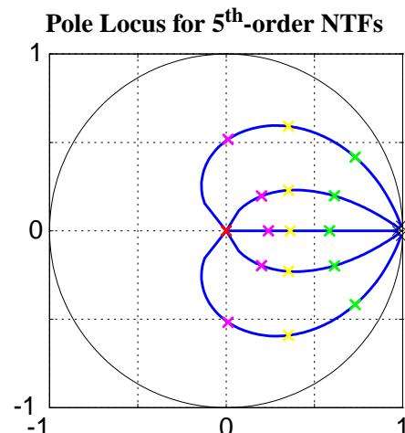
For lowpass modulators, the pole placement is similar to a Butterworth transfer function. Yields a flat STF for both lowpass and bandpass modulators employing the CRFB topology with one feed-in.
