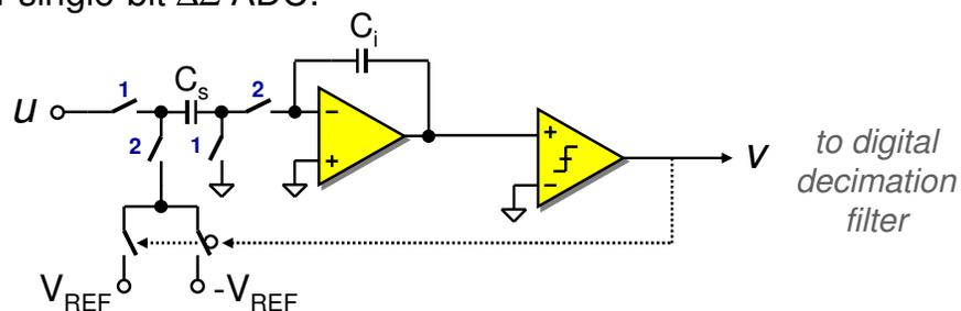
Input signal  $u$  and bitstream  $v$
