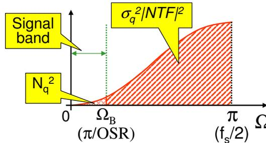
Doubling OSR increases SNR by 9 dB (1.5 bit/oct)
