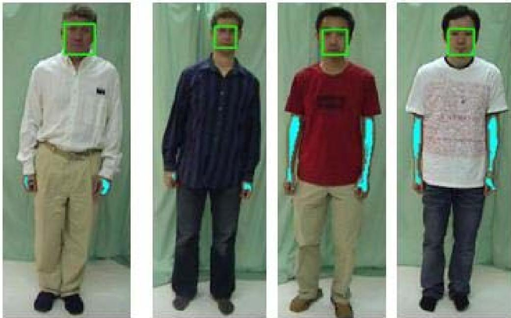
Figure 38. Examples of face detection and arm skin detection.
