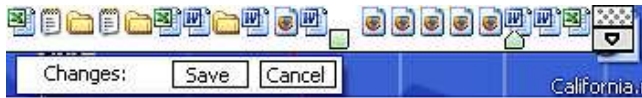
c) If a switch is changed, UI will ask for confirmation (the Save/Cancel box).
