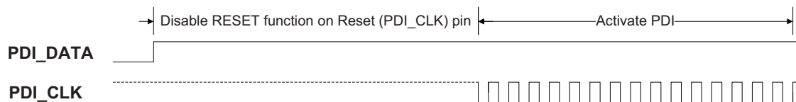
Figure 32-3. PDI physical layer enable sequence.
