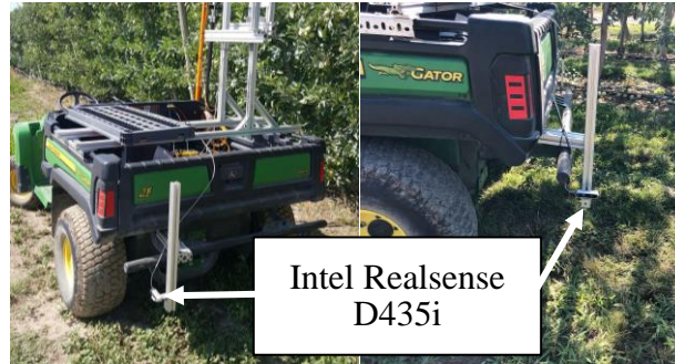
Figure 1. Utility vehicle with Intel Realsense D435i mounted near the rear at the desired height for measuring the trunk width. The camera continuously records RGB-D images as the vehicle traverses the orchard rows (Prosser, WA, USA).
