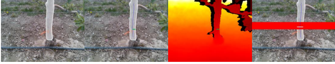
Figure 2. Left : The mask produced by Masked2Former. Middle left : The mask is processed to produce a medial axis (blue) with a distance to the boundary (an example is shown in green) at every point along the axis. Middle right : The corresponding depth image, with the green “slice” marked. Right : The pixel slices that are below the 40th percentile; the width of the largest of these (shown in white) was chosen as the trunk width.
