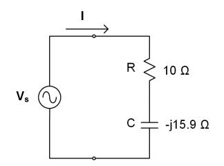
Consider the following circuit, modeling a source driving a load through a transmission line
