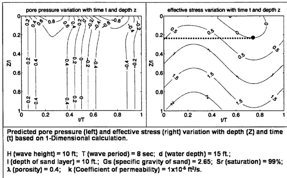
**Fig. 22.** Predicted pore pressure and effective stress variation based on 1D calculation (1 ft=0.3048 m)
