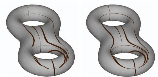
Fig. 2. Results for a height field on the original 1536-triangle mesh (left) and its subdivided version (three subdivision iterations). Note that only a source and two saddles are visible from this viewpoint.
