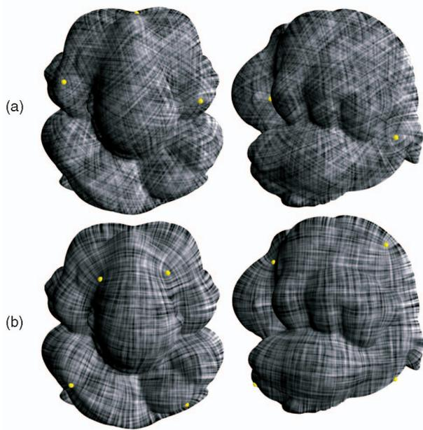
Fig. 10. The Pensatore surface is a genus-zero closed mesh. A 3-RoSy field is shown in (a), where there are six cone singularities with the curvatures of  $\frac{2\pi}{3}$ . A 4-RoSy field is shown in (b), there are eight cone singularities with the curvatures of  $\frac{\pi}{2}$ .
